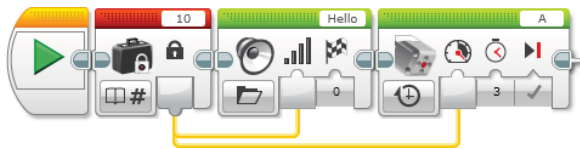
Figure 12-12: Using the Constant block to control the power of the motor and volume of the sound
