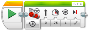
Figure 4-23: The Move Steering block on the canvas
