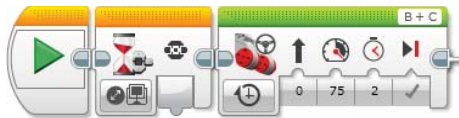
Figure 6-12: A program with the Wait block with the Compare – Brick Buttons mode
