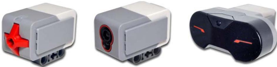
Figure 1-4: The EV3 sensors
