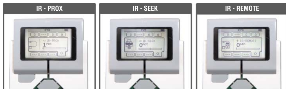
Figure 8-15: Three modes with the infrared sensor on the Port View
