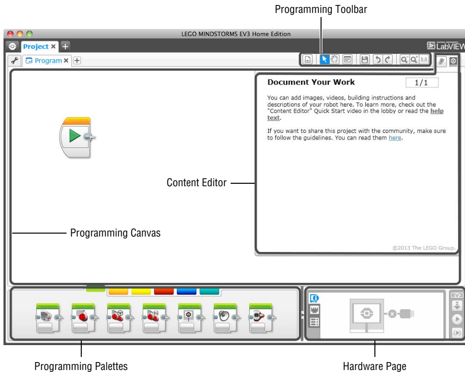
Figure 3-8: The EV3 software interface
