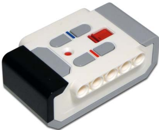
Figure 1-5: The remote infrared beacon
