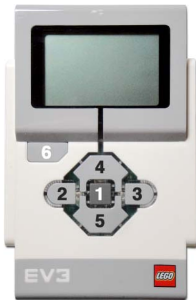
Figure 2-26: 6 Buttons on the EV3 brick
