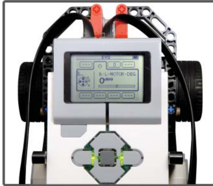
Figure 4-19: Select port B on the Auto-Driver.
