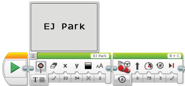
Figure 5-12: The Display block with the Move steering block; the name will remain on the screen until motors B and C make three full rotations.
