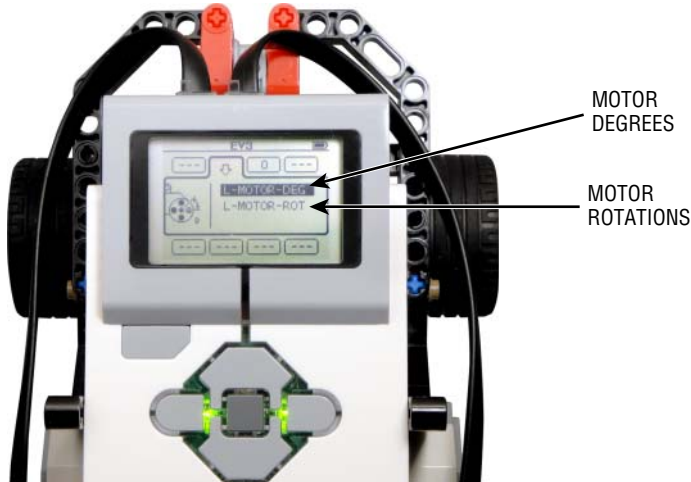
Figure 2-34: You can get two types of data from the motor: motor degrees and motor rotations
