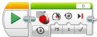
Figure 4-15: The Large Motor block on the canvas
