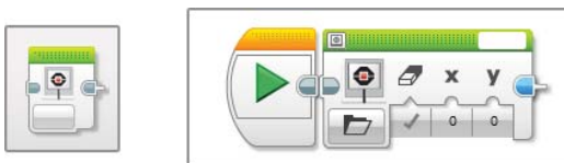
Figure 5-1: The Display block on the palette (left) and on the canvas (right)
