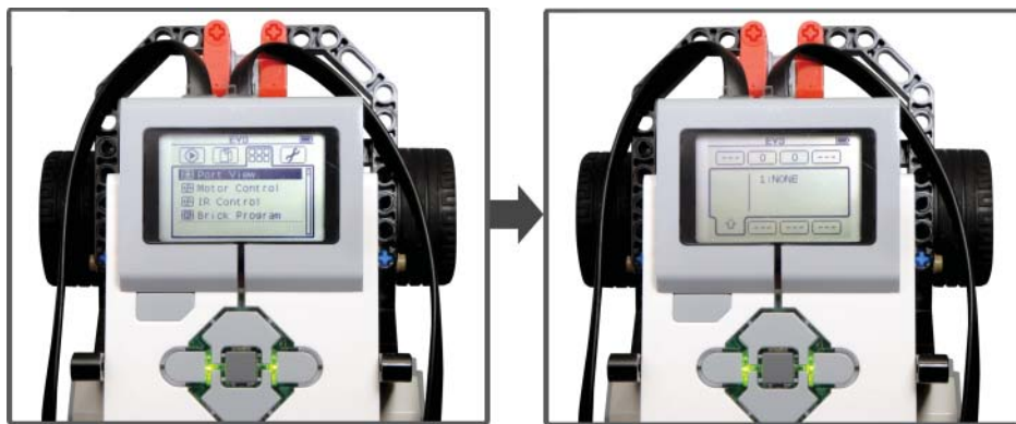
Figure 4-18: The Port View with the Auto-Driver
