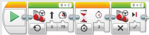
Figure 6-5: Motors B and C will be running for 3 seconds and then stop.
