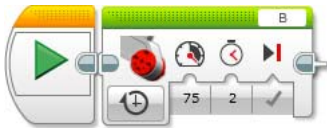
Figure 4-21: Program the left motor to go on for 2 seconds with the power of 75
