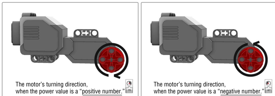
Figure 4-14: The motor Power input and the directions of the motors
