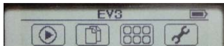
Figure 2-28: The four screen icons from left to right: Run Recent, File Navigation, Brick Apps, and Settings
