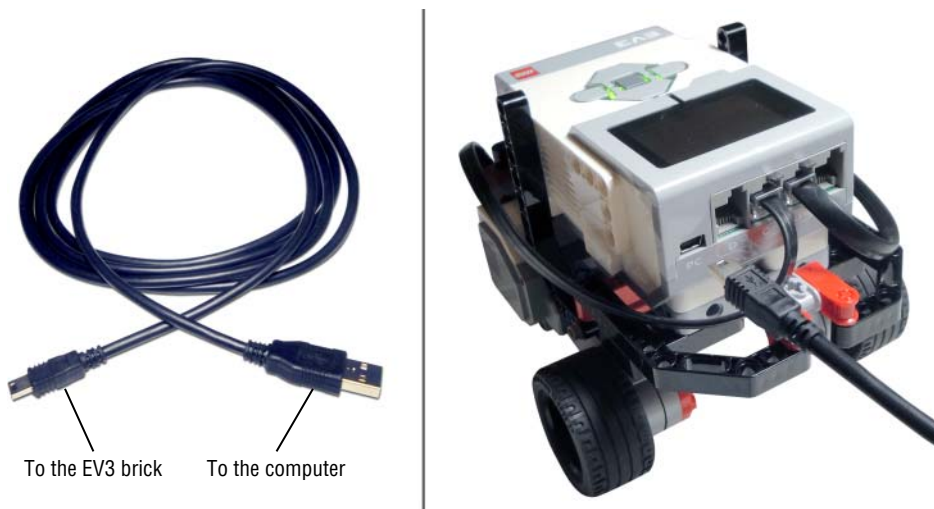
Figure 3-16: Connecting the Auto-Driver to the computer with the USB cable
