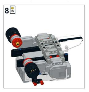
Finally, place the tires onto the hubs:
