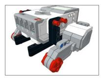
Next, we will attach wheels, skids, casters, or treads to our chassis. A robot with treads is more stable but often has a larger turning radius. The tread-based robot will also have a larger footprint. A robot with a skid or caster will turn better but only has three points of contact, and thus can tip easier.
