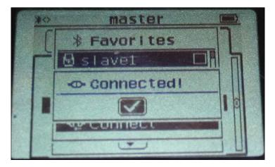
This process for connecting the robots by using the brick buttons only needs to be done once. However, if you do not do this initial pairing, when you try to execute the programs, you will receive an error.
