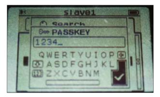
After you have entered the passkey, the robots should complete the connection. You will see the display as shown in the following image:
