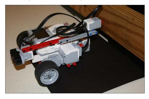
On both robots, the Touch Sensor is plugged into port 1, and the Color Sensor is plugged into port 3. The Ultrasonic Sensor is not needed for this program, but is left over from the *Maintain a distance* section's program.
