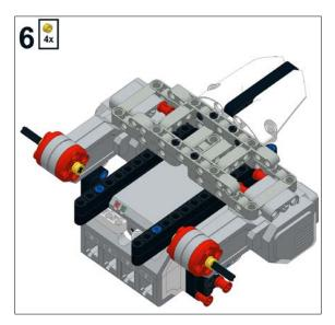
In this step, we will add the hubs for the tires. Insert the hubs onto the axles in the orientation as shown in the following screenshot:
