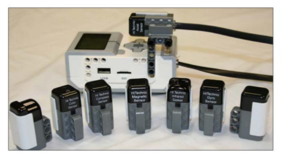
One of the most useful products HiTechnic has for the LEGO NXT MINDSTORMS are the multiplexors that allow you to use multiple sensors beyond the limit of the four sensor ports on a robot. At this point in time, they have not released the EV3 sensor blocks that will allow you to use them with the EV3. In the following image, you can see several ports for plugging in additional sensors:
