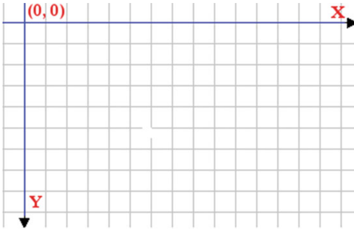
Figure 4-2. Coordinate system of LCD display
